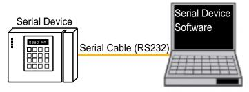
Figure 4.26 Direct Serial Connection
