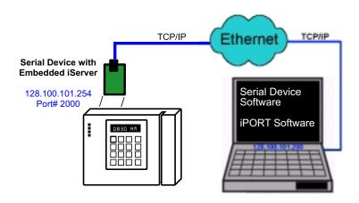
Figure 4.27 Redirect Serial Connection
