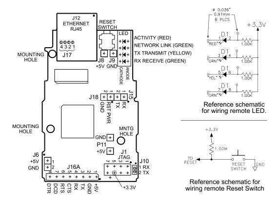
Figure 2.3 Parts of the iServer Unit
