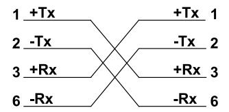
Figure 2.7 10Base-T Crossover Cable Wiring
