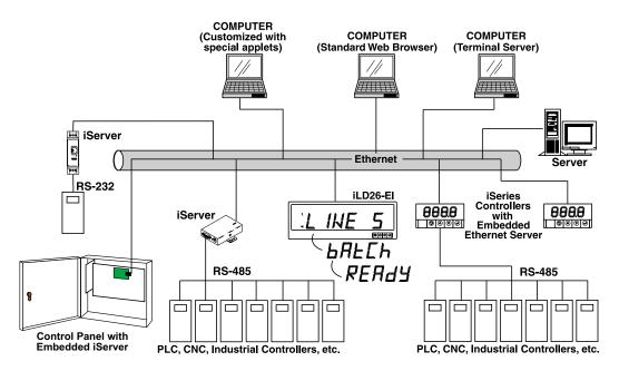
Figure 1.1 Accessing devices over the Ethernet
