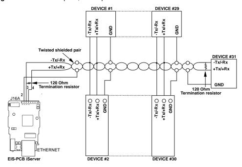
Figure 2.5 Multi-point, Half-Duplex RS485 Wiring
