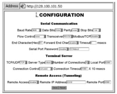
Figure 4.24 Configuration Menu - Remote iServer
