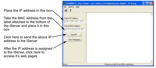
Figure 4.2 Assigning an IP Address using iCONNECT
