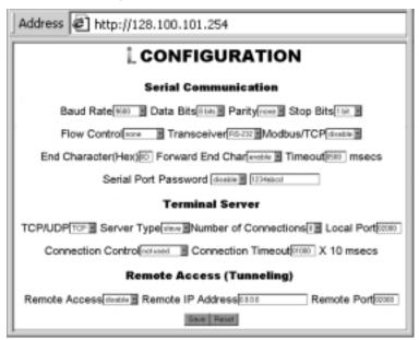
**Figure 4.18 Terminal Server Configuration**
