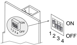
Figure 4.14 DIP switch #1 shown in "ON" position
